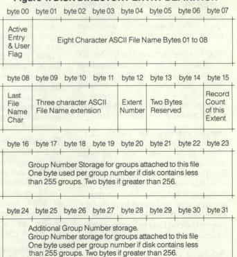
The bytes of the disk directory entry are described in the following paragraphs. The first byte stored in an entry is set to indicate whether this slot in the predetermined directory area is empty or if it describes an active file extent. A value of 0E5H indicates an empty slot. Presumably, this value was selected because a freshly formatted diskette contains all 0E5H bytes in the empty sectors, making it appear to con-
